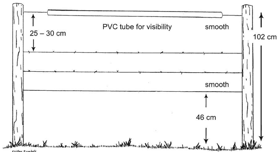
**Fig. 15.8** Design of a wire fence for containing cattle yet allowing free passage of pronghorn under the bottom wire. Note use of smooth top and bottom wires to prevent injuries. Split PVC tubing can be used to increase visibility of the top wire in high frequency crossing areas used by wild ungulates. Source: Alberta Conservation Association
